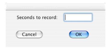
Enter the number of seconds, click OK, and Audiocorder will then start recording, and automatically stop when that number of seconds of audio has been recorded.
